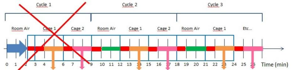
If the room air measurement duration in the first cycle is < 1 minute, room air (nor VO<sub>2</sub> calculation in each cage) will not be calculated in the cycle because the first minute is discarded, so the system will have no room air sample to calculate the reference values. Therefore, the calculations will begin with the cycle 2.
