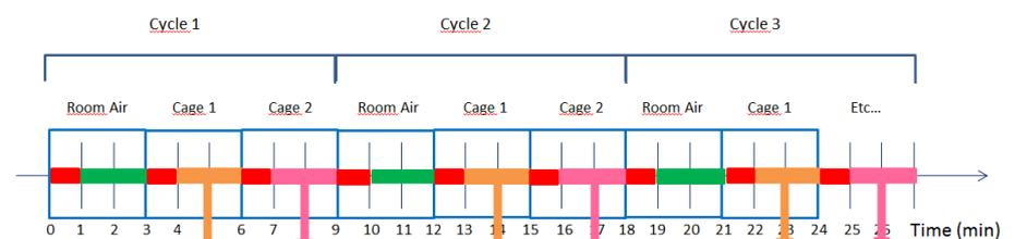
In this case, each cycle will begin with a room air evaluation and each 3 minutes, the system will switch between the cages.
