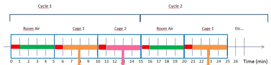
For cage 1, when the first minute is discarded, 4 minutes of samples are available for  $[O_2]$ . If the calculation interval of time of analysis is  $\geq 4$ , the system will take all the available samples (in this case 4 minutes). The same data will be obtained whether the user selects an interval of calculation of 4, 5, 6 minutes or greater.
