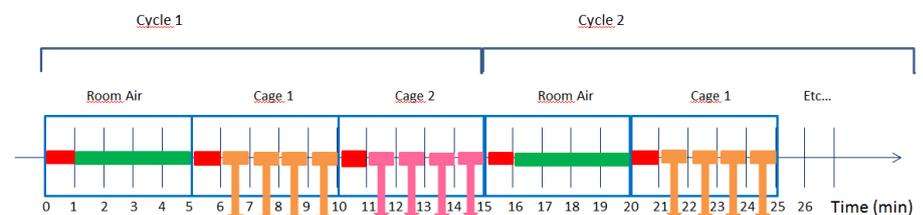
For cage 1, when the first min is discarded, 4 minutes of samples are available for  $[O_2]$ . As the calculation interval of time of analysis is 1 minutes, the system will be able to calculate four values of  $VO_2$  for each cage in each cycle. For these four calculations, the same  $[O_2]$  in room air will be considered (average of all the available samples available after subtracting the first minute).
