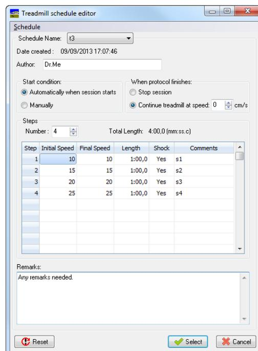
METABOLISM allows very flexible control of the treadmill belt speed in the range of 5 to 150 cm/sec from the Protocol definition procedure. A value of 0 cm/sec halts the belt movement.
