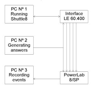
The following is the structure of the validation set-up:
