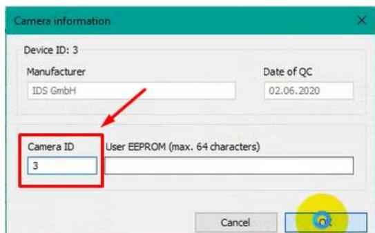
11. Connect the next camera and repeat the step until all the cameras have been connected and set with an appropriate ID.
