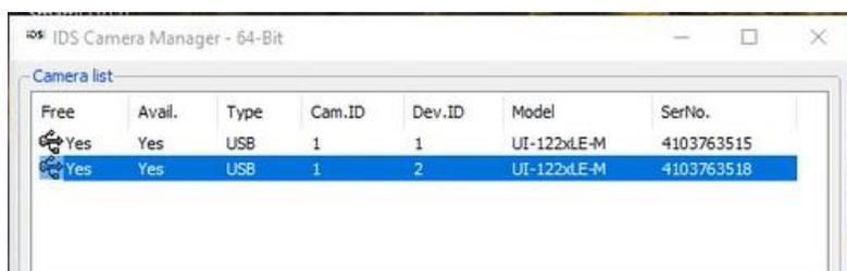
5. The IDS Camera Manager displays the camera Serial Number (SerNo.) as well as the Camera ID (Cam.ID) and Device ID (Dev.ID). The IDS Camera Manager always sets the Camera ID (Cam.ID) to 1. The Cam.ID should be changed to 2.
