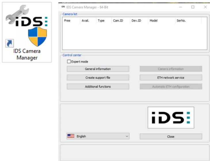
2. Connect the first camera. If a USB HUB is needed to connect multiple cameras to the computer, make sure that you connect the camera first to the USB Hub and then USB HUB to the computer. The camera will be automatically detected by the IDS Camera Manager and displayed in the Camera list.
