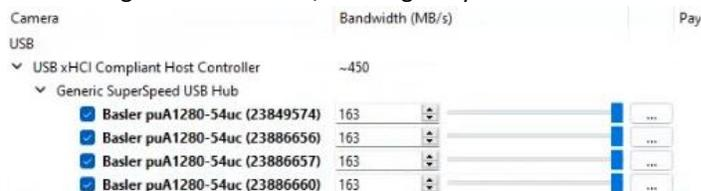
Divide 450 MB/s by (4+1) = 5 cameras (total 90 MB/s) and modify the bandwidth per each camera.
