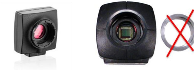
1. Unpack the camera, remove the O-ring from the objective and mount the lens. If the O-ring is not removed, the image received from the camera may be blurry. This ring may be black or silver in color.
