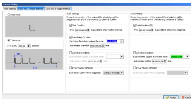
A train of 50 ms pulses given at specific intervals (period time, TP) is triggered whenever one of the selected start conditions is fulfilled. The available start conditions are the same previously explained for Pulse mode. The train of pulses is stopped when the selected stop conditions is fulfilled:
