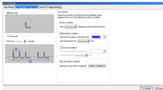
A unique 50 ms pulse is triggered whenever one of the selected start conditions is fulfilled:
