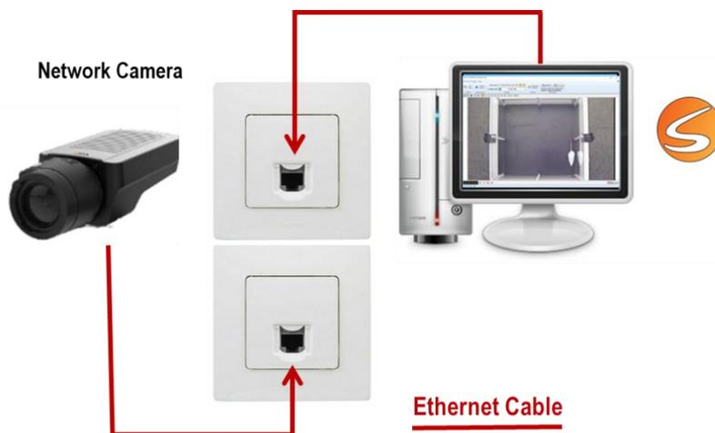
It is possible to connect up to 16 cameras simultaneously. However, be aware that you will need an Ethernet Switch POE to connect more than one camera at the same time.
