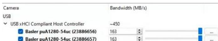
If the sum of the bandwidth of all the cameras exceeds the bandwidth of the USB controller, divide this last value for the total number of cameras + 1.
