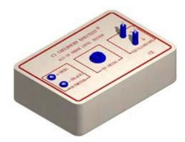
The A13-16 Shock Level Tester allows for verification of the shock output of a shock source. This unit requires a Volt Meter and/or Oscilloscope (not included). The input jack connects to alligator clips (included) that can easily be attached to either subject electrodes or the grids of the shock floor.
