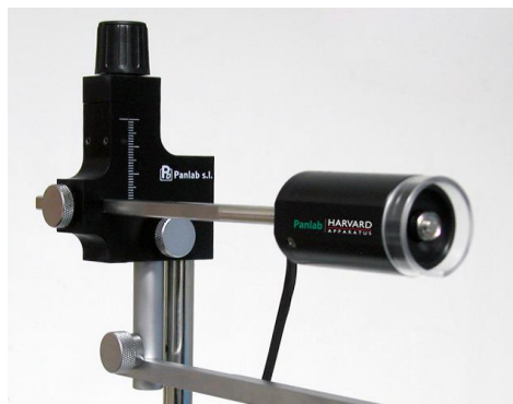
Figure 24. Micropositioner/ Tissue Holder/ Transducer Assembly.
