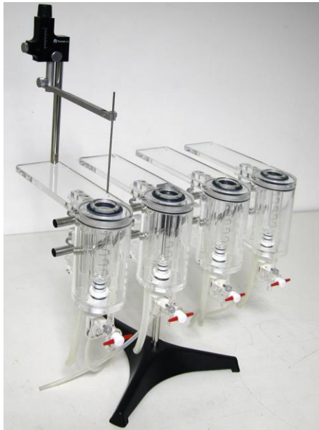
Figure 1. Four module LE 11100 Organ Bath assembly.
