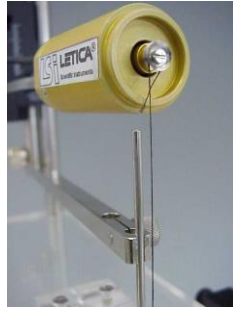
Figure 22. Fixing the Tissue to the transducer.
